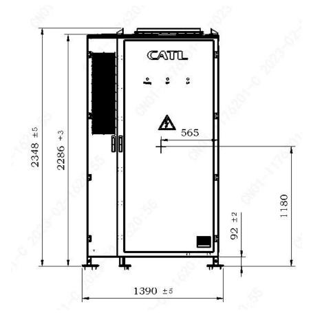
Figure 15 The Front View and Dimensions of EnerOne+
