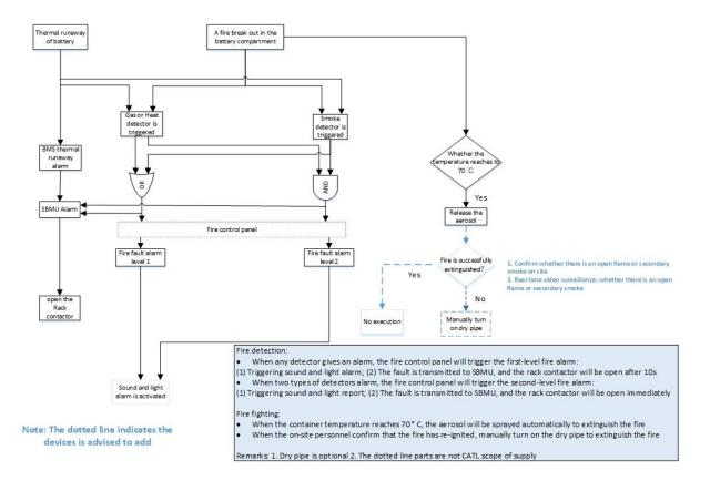
Figure 6 Control logic of FSS
