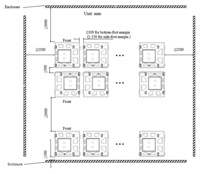
Figure 13 Layout of the rack
