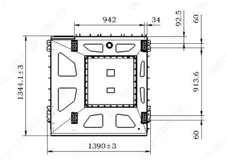
Figure 17 The Top View and Dimensions of EnerOne+
