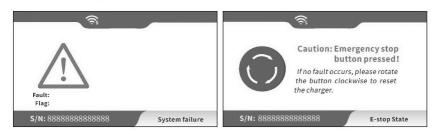
Fig. 6-4 Display of fault state
