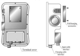
Fig. 5-4 Fix the wall-hanging accessories
