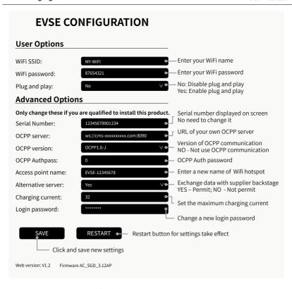
Fig. 6-8 Set parameters to config the Sunnic
