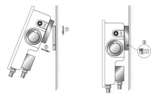
Fig. 5-7 Fix the wallbox on the wall
