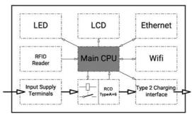
Fig. 4-2 Block diagram of products
