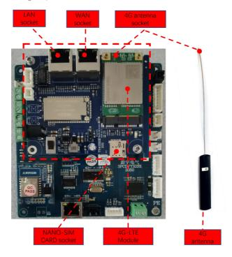
Fig. 5-8 4G PCBA in the charging station
