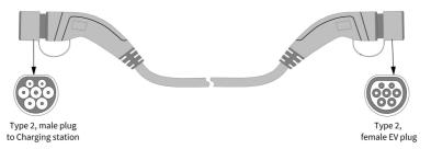
Fig. 3-4 Dual-connector charging cable
