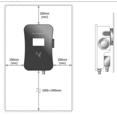
Fig. 5-2 Minimum space requirements for wall mounting
